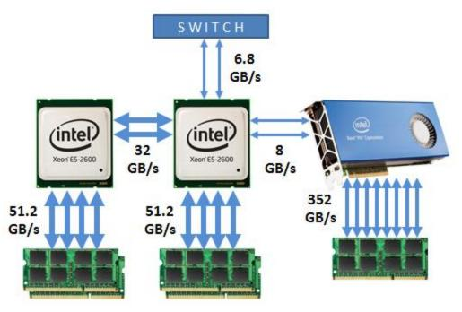
The MIC is like another node on the IB network, with its own OS, own internal memory, and own external IP address
